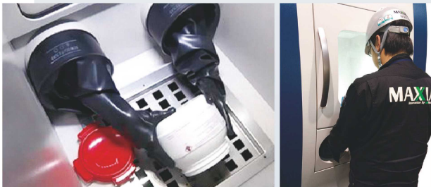
Powder supply (APR system inside)
